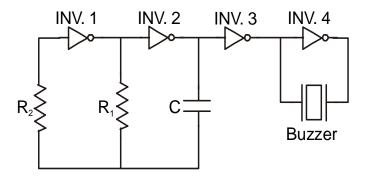
Figure 106: Inverter Push-Pull Circuit
