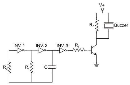
Figure 107: External Drive Circuit Using A Transistor
