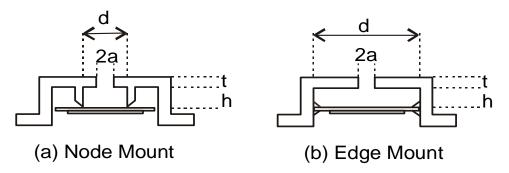
Figure 103: Cavity Measurements For Helmholtz's Formula
