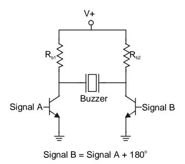
Figure 108: External Drive Push-Pull Circuit
