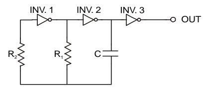
Figure 105: Example of External Drive Circuit
