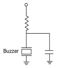
Figure 110: Capacitor Bypass of Buzzer
