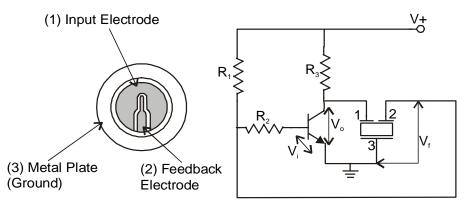
Figure 109: Example of Self-Drive Circuit
