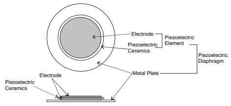
Figure 100: Piezoelectric Diaphram
