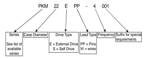
Figure 111: Buzzer Part Number System
