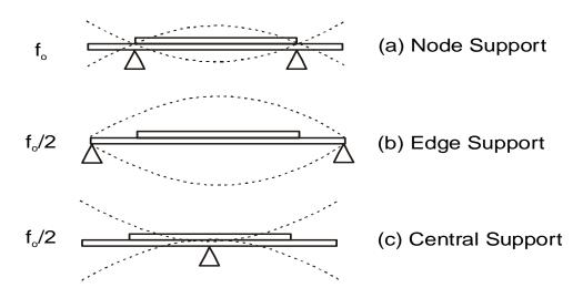
Figure 102: Mounting Methods
