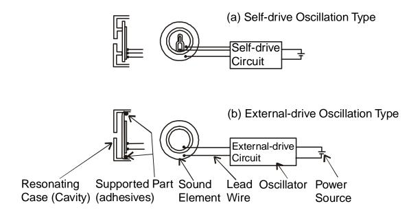
Figure 104: Two Drive Oscillation Types
